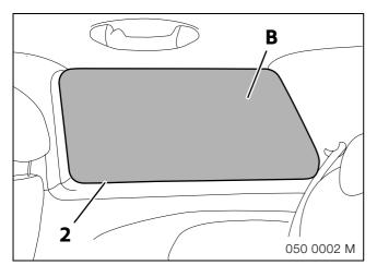
Apply sun guard film **B** to the window (2), aligning it to precisely fit the window on all sides.
