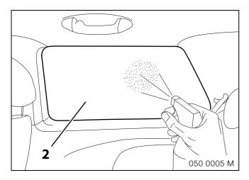
Spray the window (2) where the film is to be glued with assembly fluid **E**.
