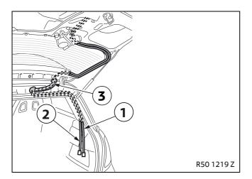
Route sensor cables (1) and (2) along the standard wiring harness through the grommet (3) and into the right-hand side of the trunk.
