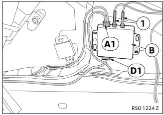
Connect the sensor cable (1), branch **A1** (SW 4-pin) and branch **D1** (SW 4-pin) to control unit **B**.
