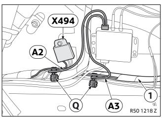
Route branch **A2**, SW cable, to joint connector **X494**, BR cable, and connect it with miniature connector **Q**.
