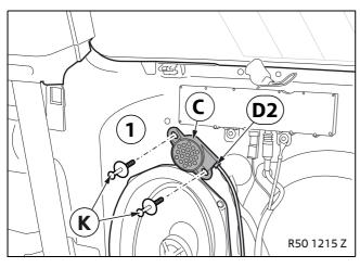
Place signal generator **C** on the right body side section (1) and mark the positions for the holes.
