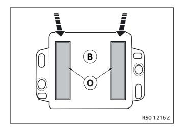
Clean and degrease the gluing surfaces.
