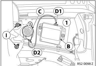
Place the signal generator **C** on right-hand side of the boot (2) and mark the positions for the holes.
