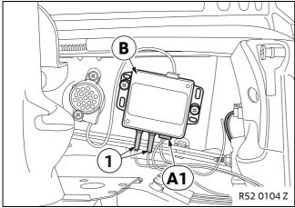
Connect the sensor cable (1) and branch A1 (4-pin SW) to control module B.
