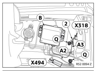
Route branch **A2**, SW cable, to joint connector **X494**, BR cable, and connect it with a miniature connector **Q**.
