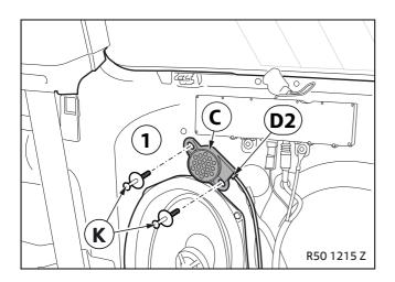
Place the signal generator **C** on right body side section (1) and mark the positions for the holes.
