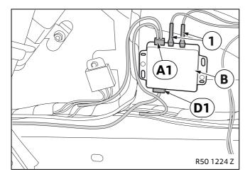
Connect the sensor cable (1), branch **A1** (4-pin SW) and branch **D1** (4-pin SW) to the control module **B**.
