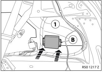
Affix the control module **B** to the side part of the body (1) using Velcro strips **O**.
