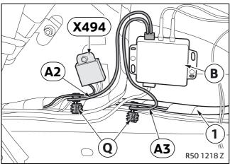
Route branch **A2**, SW cable, to joint connector **X494**, BR cable, and connect it with a miniature connector **Q**.
