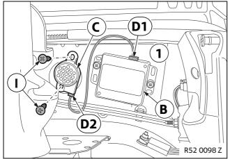
Place the signal generator **C** on right-hand side of the boot (2) and mark the positions for the holes.
