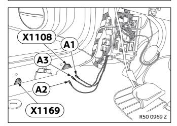
Connect branch A1, BR cable, and branch A2, WS/SW cable, to the joint connector X1108, BR cable.
