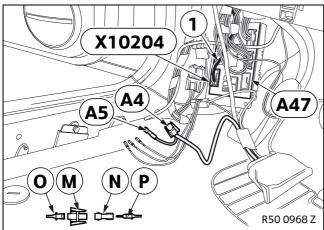
Connect branches **A4** and **A5** to plug **X10204** (natural-coloured 12-pin) on fuse holder **A47**:
