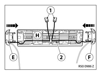
Plug right sensor **E** and left sensor **F** into the registration plate holder **H**.
