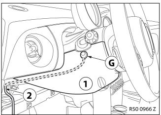
Clean the bottom steering column casing (1) and affix the button **G**.
