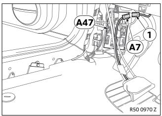
Connect branch A7 to the connection cable (1) for button G.
