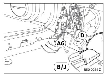
Connect branch **A6** and the signal sensor cable **D** to the control module **B**.
