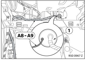
Thread branches **A8** and **A9** through the grommet (1) into the engine compartment.
