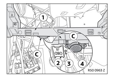
Place the signal generator **C** on to the instrument holder (1) next to the OBD socket (2) as shown.
