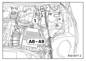
Cut into the cover (1) and make a hole for the cable passage.
