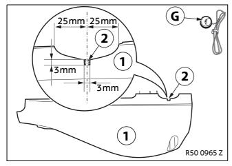
Mark the specified dimensions on the lower steering column trim (1).
