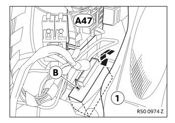
Place the control module **B** between the fuse holder **A47** and the carpet (1).
