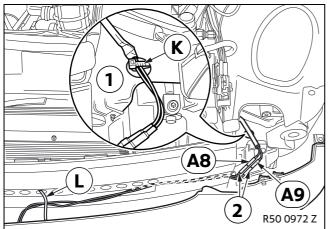
Use a 6 mm twist drill bit to drill through the inner wing (1) at a suitable point and push in cable tie holder  $\mathbf{K}$ .
