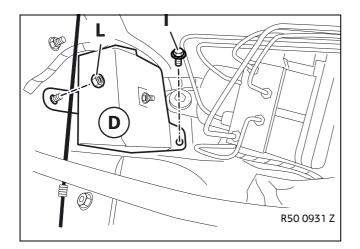
Use a hexagonal screw  ${\bf I}$  and hexagonal nut  ${\bf L}$  to secure the emergency-current siren holder  ${\bf D}$ .
