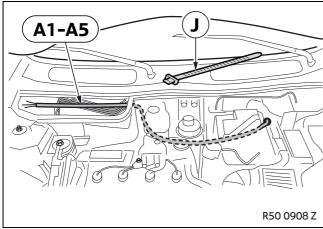
Make sure that connection cable A does not come into contact with the wiper linkage.
