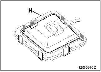
Note the installation direction, the arrow on ultrasonic module holder **H** must point towards the front of the car. ◀
