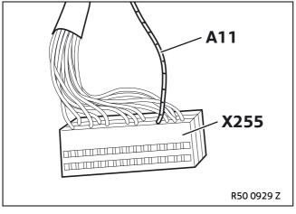
Connect branch **A11**, GR/SW/GE cable, to PIN 14 in plug **X255**.
