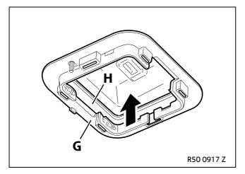
Note the installation direction, the arrow on ultrasonic module holder **G** must point towards the front of the car. ◀
