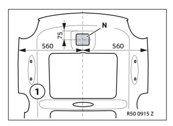
Position the template **N** on the raised area in the centre of the installed headlining (1).
