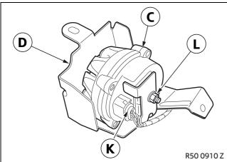
Use a hexagonal nut **L** to secure the emergencycurrent siren **C** to the holder **D**.
