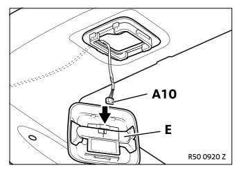
Connect branch **A10** to the ultrasonic module holder **E**.
