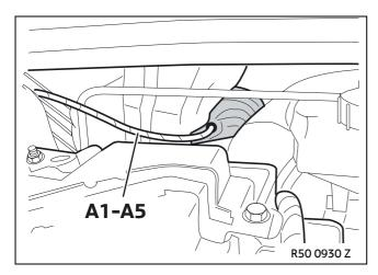
Thread branches **A1-A5** through the cable grommet on the driver's side.
