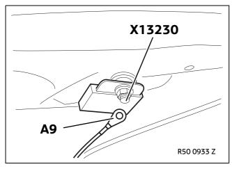
Screw the cable eyelet A9 to earth bolt X13230.
