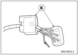
Connect branches **A1-A5** to socket casing **K** as follows:
