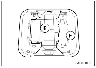
The installation arrows on ultrasonic module **E** and ultrasonic module trim **F** must point towards the front of the car. ◀
