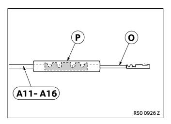
If branches A11-A16 do not fit into plug X253 or X255, use the butt-joint connector and shrink hose P to install the supplied repair cable O.
