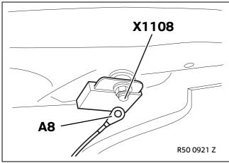
Screw the cable eyelet **A8** to the earth bolt **X1108**.
