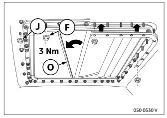
The inside of the outer roof panel can be taped over with cardboard, which must be removed so that the correct seating of the rails is not affected.
