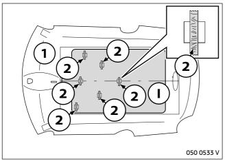
Provisionally secure template for headliner I with adhesive tape (2) on the top of headliner (1).
