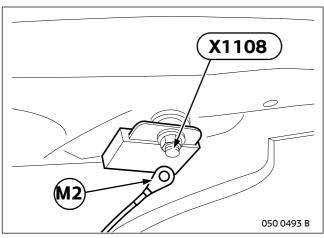
Connect junction **M2** to earth point **X1108** in front part of left-hand sill.
