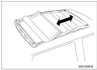
Move folding sunroof  ${\bf A}$  to the front or rear until the folding sunroof  ${\bf A}$  is correctly seated.
