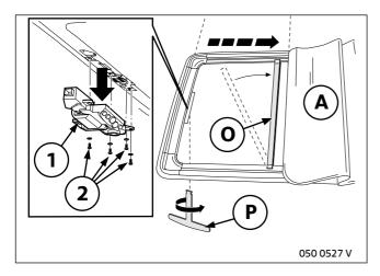
Completely open folding sunroof **A** with hand crank **P** by turning folding sunroof motor (1).
