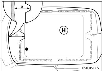
Align template for outer roof panel **H**, centralise and fix it in place with adhesive tape.
