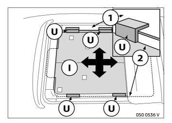
Place centring angles **U** (4 pcs) on folding sunroof frame (1) and template for headliner **I** on centring angles **U** on line (2), as illustrated.
