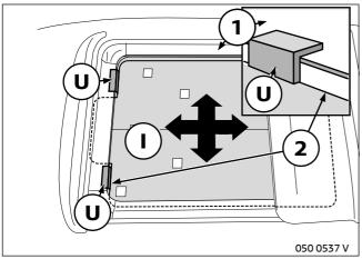
Place centring angles **U** (2 pcs) on folding sunroof frame (1) and template for headliner **I** on centring angle **U** on line (2) as illustrated.
