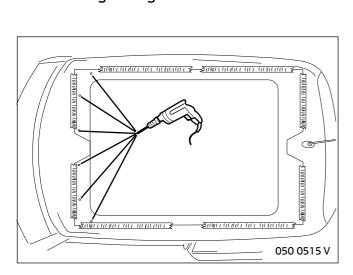
Drill 6 securing holes with ø 7 mm on template for outer roof panel **H** for wind deflector **K**.
