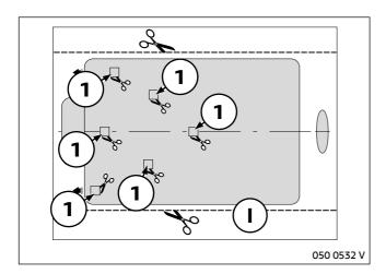
Cut out template for headliner I along the dotted line. Also cut out holes (1) in template for headliner I.
