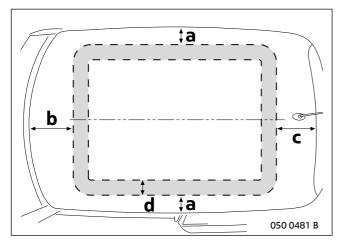
Attach masking tape to the shaded area in the illustration.
