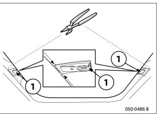
Cut out the rest of the roof brace (1).
