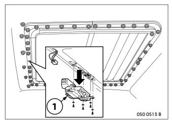
Once the function check has been completed, disconnect and remove folding sunroof motor (1).
