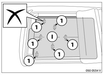
Remove adhesive tape (1) from template for headliner I again.
