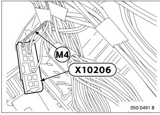
Plug junction **M4** into **PIN 1** of the green, 12-pin socket housing **X10206**, on the fuse box.
