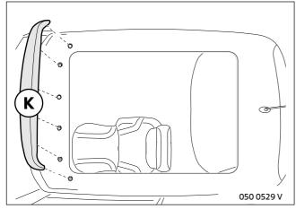
Remove protective film from double-sided adhesive tape on the underside of wind deflector **K**.
