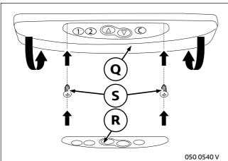
Clip in trim piece for folding sunroof motor **Q** and secure with two screws **S**.
