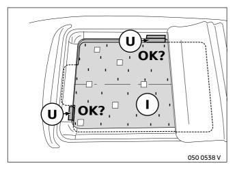
Before tacking template for headliner I check again with centring angle **U** that template for headlining I is correctly located on the headlining.
