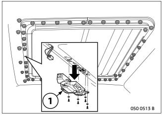
Once the function check has been completed, disconnect and remove folding sunroof motor (1).
