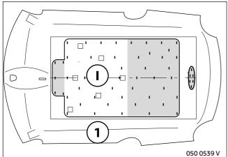
Tack template for headliner I onto the shaded area of the headliner (1).
