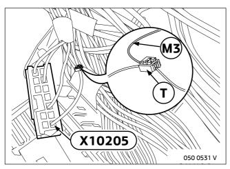
Connect junction **M3**, wire colours RT/BL, with mini-connector **T** to GN/BL wire from **PIN 12** of blue, 12-pin connector **X10205**.
