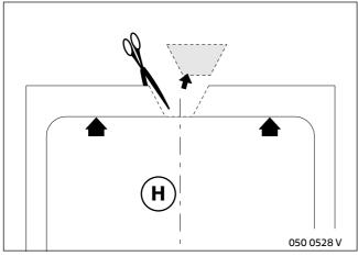
Cut out template for outer roof panel **H** a t the front end along the dotted line.
