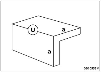
Both edges of centring angle **U** have a length of a = 30mm. ◀
