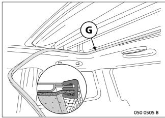
Starting in the middle, route weatherstrip **G** along the inside edge of the folding sunroof and headlining aperture.
