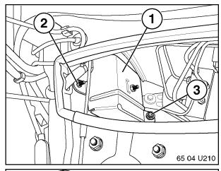
Install siren-tilt sensor/bracket assembly (1) in place and secure with M6x12 hex bolt w/captive washer (3) and M6 hex nut w/captive washer (2) as shown.
